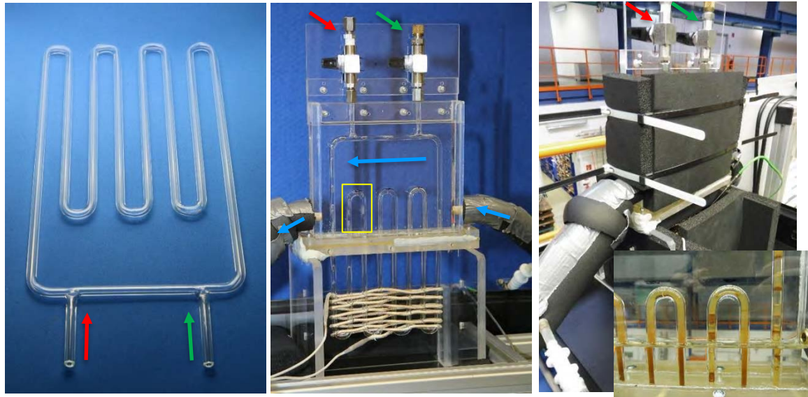
Figure 1. Oscillating heat pipe – Test rig. Left glass body of OHP, centre not insulated test rig filled with DI-water (yellow rectangle highlights slug-bubble formation of working fluid) and right insulated test rig with inserted photo of slug-bubble formation of ferronanofluid. Connecting pieces for evacuation and filling are indicated by red and green arrows, flow through condenser by blue arrow.
